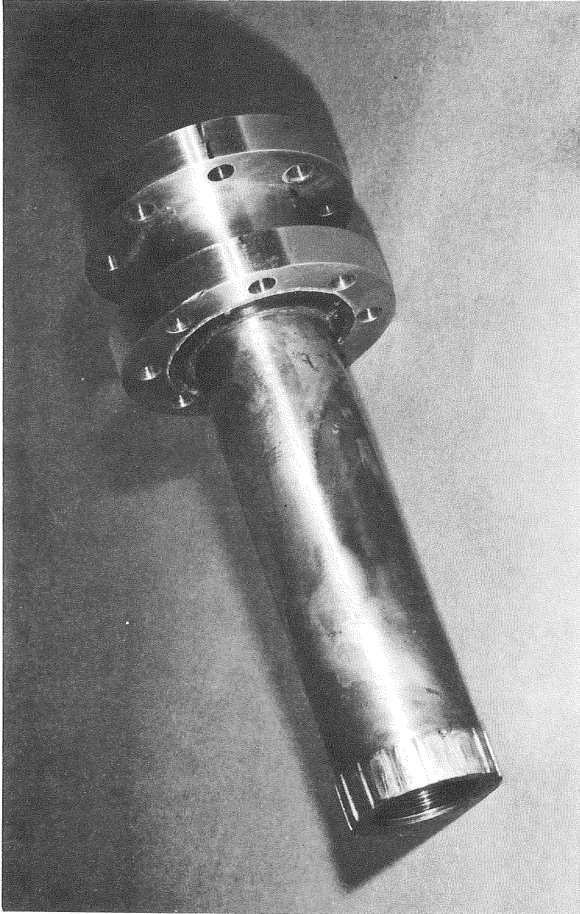
5AA33-10/11/65-SIC Figure 14. Photographic Representation of the Catalytic Igniter Used in the Parametric Engine Evaluation Task
